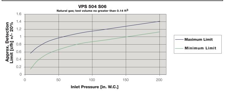
**NOTE**: Leak detection limit depends on inlet pressure and gas density. To obtain detectable leakage through both valves, divide values in graph by 1.6.
